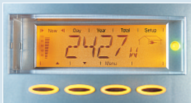
The Fronius Personal Display shows current data from up to 15 inverters.
