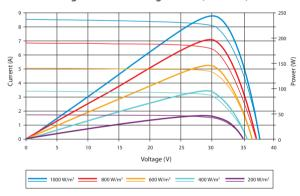
Exellent performance under weak light conditions: at an irradiation intensity of 200 W/m² (AM 1.5, 25 °C), 95.5% or higher of the STC efficiency  $(1000\,\text{W/m}^2)$  is achieved
